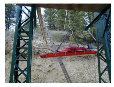
folded and tied to contain one meter of slack that could be instantly loosed to simulate the drop. The CTM 200 as tested weighed 19 lbs and was loaded with a Rescue Randy weighing 173 pounds for a total weight of 197 pounds. The litter was hoisted up a drop tower for the test.
