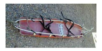
right railing brackets at the nose were pulled from the shell and one end of the litter railing sheared from the FastLock<sup>TM</sup> System. It was observed that the litter was still in one piece and could be considered functional although patient integrity could have been compromised. It was also observed that the railing of the litter was the cause of central failure due to buckling.
