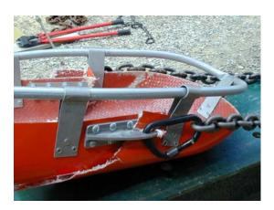
TEST SIX - CTM200 Litter Railing Bracket Pull Out
