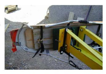
the bracket closest to the carabiner. At this point, the litter, while badly damaged was still attached to the litter harness by three of four attachment points. After several more seconds it was determined the litter had sustained enough damage to render it inoperable. Absolutely no damage was done to the <sup>1</sup>Fastlock<sup>TM</sup> System and the remnants of the litter were disassembled at the completion of the test.
