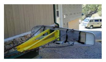
A rigid backboard was manufactured to place in the bottom of the litter to distribute the load of the SPD across the length of the litter. The footprint of the backboard was 60 inches by 11.25 inches. The distance from the center of the ram to the end of the litter was 47.25 inches and from the head of the litter to the ram was 34.75 inches.
